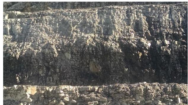
*Figure 3 Presplit Results Using Emulsion based Presplit*
