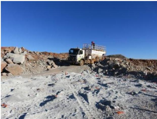
Figure 3 NSA's versatile MPU (17T Road Legal with Trailer)
