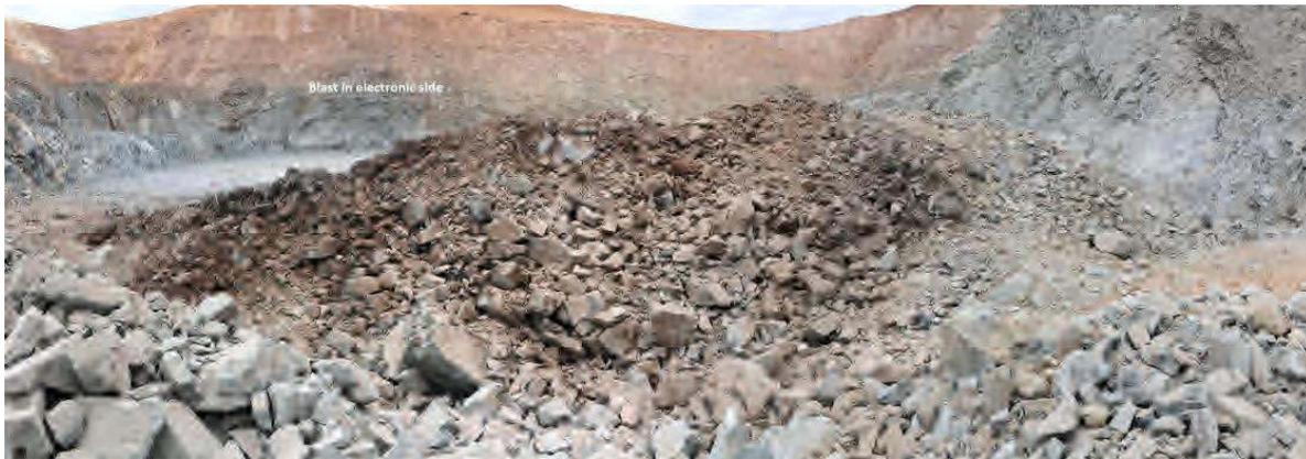
Figure 8 Blast Fragmentation NSA Bulk Explosives Trial 2\_ Electronic Section
