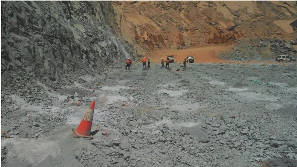
Figure 10 Presplit Wall Surface (Left Hand Side of Screen)
